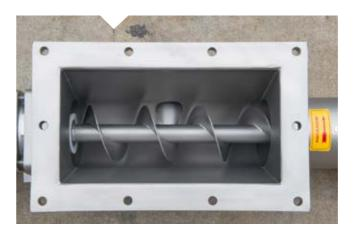
2.5" 6 bar progressive cavity pump with VSD, stand and pre-feeding screw. Single stage 1.1 kW, 54rpm (pump and motor only).
