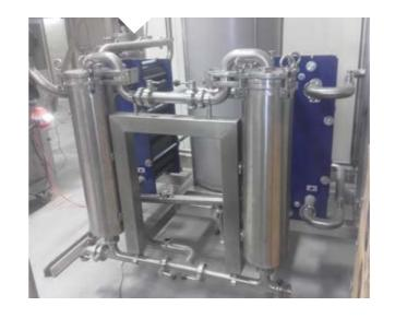
2" size 2 top entry short bag filter to fine filter honey. Includes long displacement torpedo and leg set. 0-10 bar manual pressure gauge.
