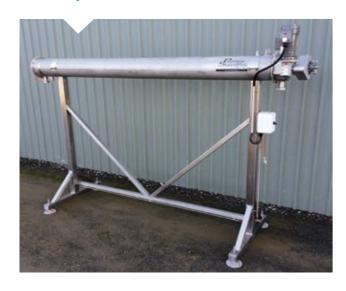
Multi tube heat exchanger to boost honey temperature prior to wax separation. 26 tubes with a powered scraper, 3500mm long, and digital temperature display to process 1250kg per hour. Constructed from stainless steel with 10-amp single phase plug.
