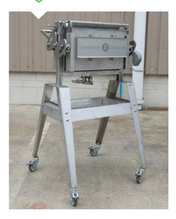
Loosen honey in full and ¾ honey frames. Hand powered operation and suitable for viscous honey. This machine is quiet and easy to operate with an innovative clean design. Constructed from stainless steel and mounted on a mobile stand.
