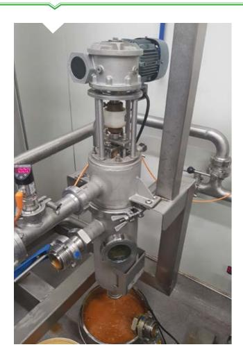
2" rotary self-cleaning wedge wire filter – to filter contaminants from honey with reduced pressure. o-10 bar manual pressure gauge with manual dump valve, three phase power (excludes electrical control).
