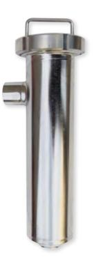
Static wedge wire to coarse filter honey – right angle filter. Constructed from stainless steel.
