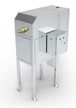
$\label{thm:contact} \mbox{Horizontal centrifuge to separate wax from extracted honey}.$ Closed circuit separation, variable speed drive, not suitable for use with un-capper. Constructed from stainless steel with 15-amp single phase plug.
