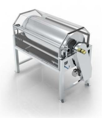
CrystechNZ external scrape surface heat exchanger to cool honey down after flash heating. 45-20° cooling at 1200kg per hour. Includes control box with variable speed control. Constructed from stainless steel with 10-amp single phase plug. Excludes cooling water supply.
