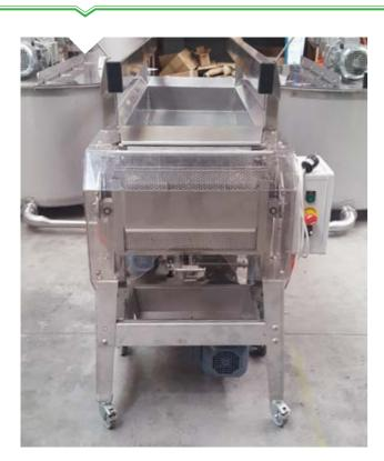
Loosen honey in full or ¾ honey frames – suitable for viscous honey. This machine is quiet and easy to operate with an innovative clean design and air powered operation. Constructed from stainless steel and mounted on a mobile stand with 10-amp single phase lead. Compressed air required.
