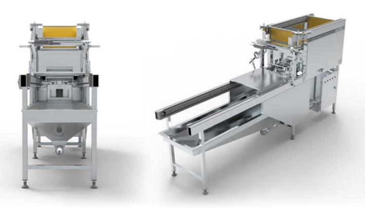
Loosen honey in full and ¾ honey frames with powered infeed and outfeed chain conveyors. Automatic start and continuous cycle operation with integrated honey sump. Integrated honey sump to fit with pump 1-101-01-01-00 (pump excluded). Constructed from stainless steel with 10-amp single phase lead. Compressed air required.
