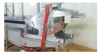
Cut back honey comb from honey frames at up to 11 frames per minute. Constructed from stainless steel with single phase 10-amp plug.
