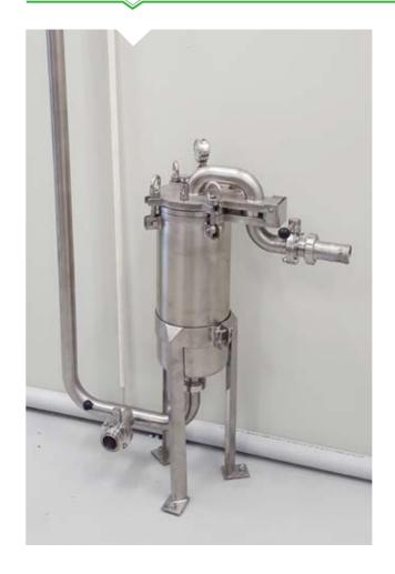
2" size 1 top entry short bag filter to fine filter honey. Includes short displacement torpedo and leg set. o-10 bar manual pressure gauge.
